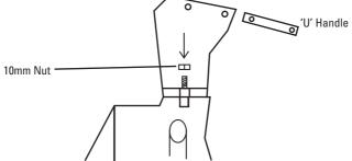
7. Attach the 'U' handle to the hopper sides using the four M8x40 bolts provided (Nyloc nuts inside hopper).
