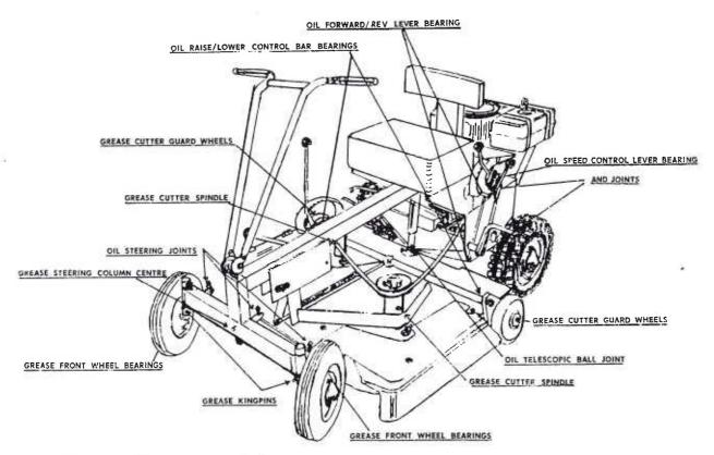
LUBRICATION POINTS (COVER REMOVED)
